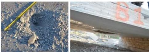
**10.5 kg** – 5 explosive cartridges. Slab fully breached.
