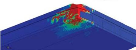
Pressure and damage profiles on top and bottom surfaces confirm the occurrence of two distinct failure modes.
